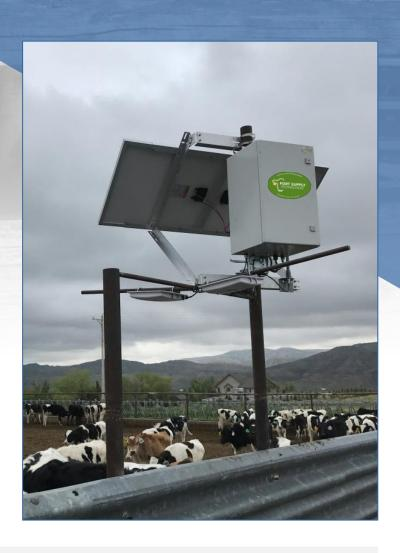
This autonomous health monitoring system utilizes UHF technology to track individual cattle activity patterns to and from their water source, applies a proprietary algorithm for early sickness detection, and alerts your team to take action sooner.
